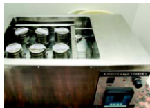
Pasteurisation in Shaker Water Bath by Pretoria Holder Method at 63°C for 30 min
